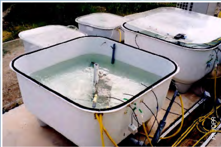
Experimental setup for the study of carbon dioxide absorption by the marine microbial communities: bacteria, microalgae, etc.
