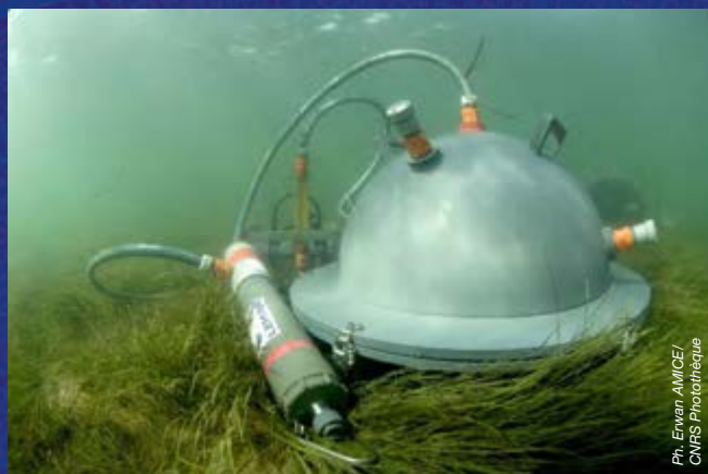
Breathing experimental chamber of a Zostera noltii seagrass meadow in the gulf of Banc d'Arguin (Mauritania). The aim? To measure the oxygen production and the carbon dioxide flux. More broadly, the aim of the PACOBA project is to enhance our knowledge of the biocenoses - the plant and animal populations - of this coastal region.
