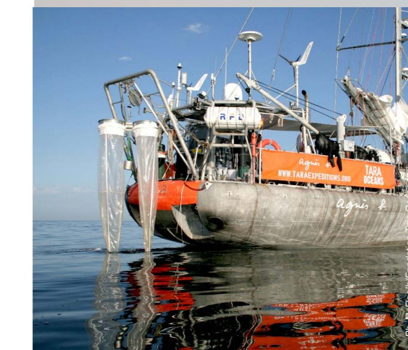
Deployment of a Bongo type net - Its dimensions and its filtration capacity make it an effective tool for searching for rare species, in particular the eggs and larvae of fishes.
